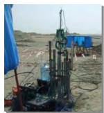
600mm pile under test
